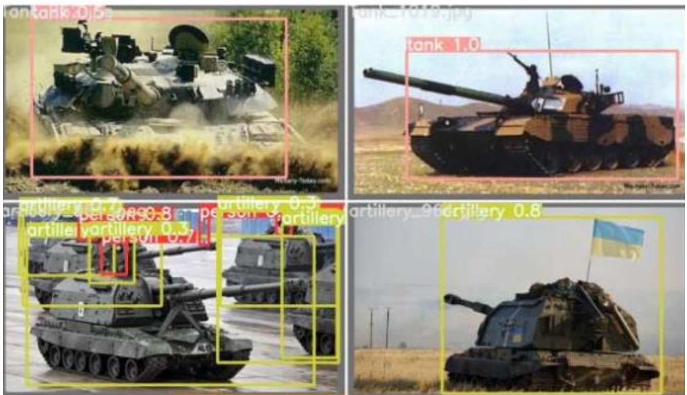
Figure 5. Ability of detecting military target using YOLOv5 enchanted with PANet.
